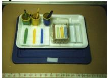
A jig shows the layout of materials in their correct sequence in Figure 2.
